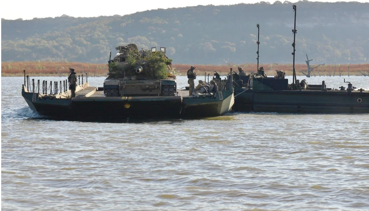
Figure 1. 1/1CD rafting their Armored Cavalry Troop during Remagen Ready 24-01 – An M1 Abrams tank rides on a 43 rd Multi-Role Bridge Company (MRBC) raft under the direction of 2-8 Cavalry and the 20 th Engineer Battalion. Rafting operations took place after 2-5 Cavalry had seized far-side objectives via air and boat assaults. (U.S. Army photo by MAJ Garrison Spencer, U.S. Army Corps of Engineers (USACE) Public Affairs Officer)
