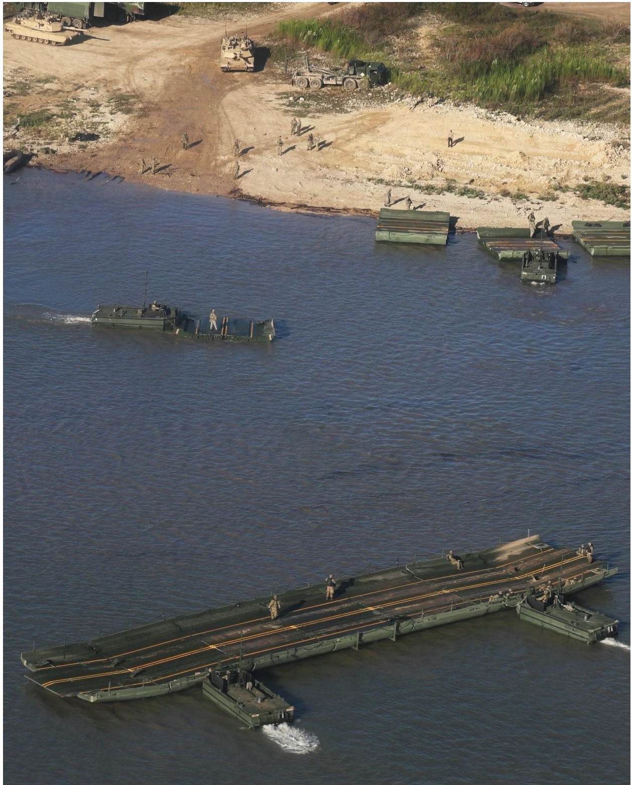
Figure 2. Multi-Role Bridge Company Raft Construction – The 43 rd and 74 th MRBCs assemble 7-Float rafts capable of ferrying multiple armored vehicles across Belton Lake. Early trips are conducted using a horizontal rafting style (pictured above), while subsequent iterations employ longitudinal rafting where the Bridge Erection Boats are positioned on both sides of the raft. (U.S. Army photo by MAJ Garrison Spencer, USACE Public Affairs Officer)
